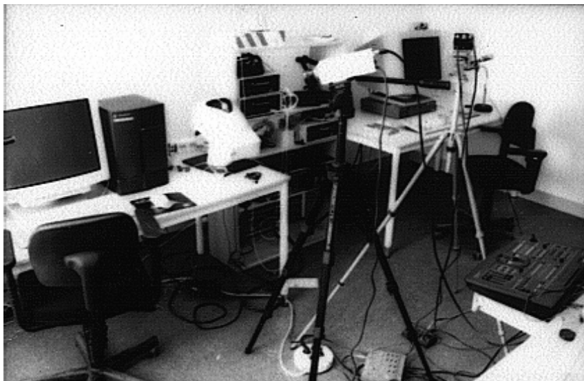
Figure 14: The hardware setup: two SGI workstations, with one camera on each for recording.
